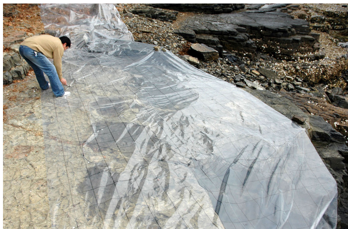
Fig. 3. Mapping and measuring directly on the field using a large transparent vinyl sheet enough to cover the whole trackway.
